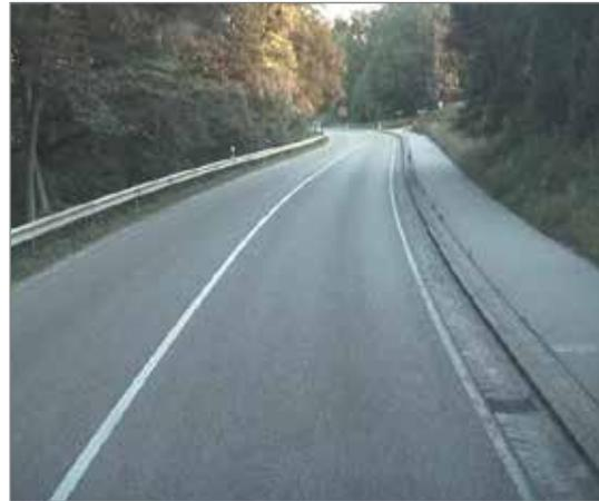
The solid line centre road marking makes the course of the road and the lane limits clearer. In addition, overtaking is banned.
