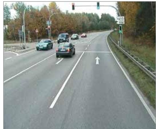
Traffic lights with separate left-turn phase clearly separates the traffic flow and ensures fast and safe turning.
