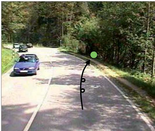
The road layout was discontinuous. In addition, there were trees at the edge of the road. The direction of the bend was hard to see, which promoted single-vehicle accidents that had severe consequences where vehicles collided with the trees.
